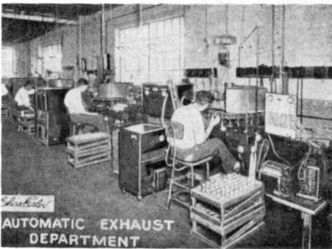
Making radio tubes in 1928 with Eisler automatic exhaust machines in the Tate factory in Irvington, New Jersey.
